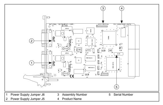
Figure B-3. PXI-8461 Part Locator Diagram
